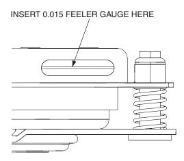
Figure 6-11. Clutch Air Gap Adjustment
